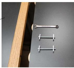
Lay up right section. Bolt the 2 sections together with the draw bolts shown
