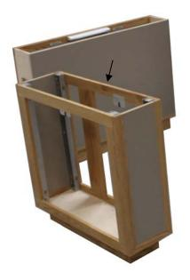
Bolt corner posts on face frames to base with 7/8 x 1/4 x 20 hex head bolts
